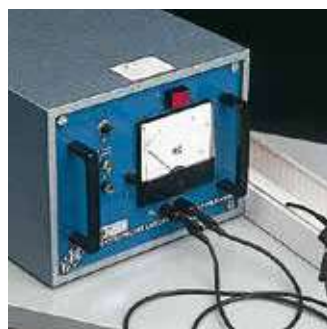
Apparatus for insulation resistance above 100 MΩ.
