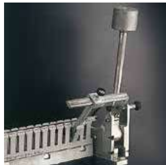
Apparatus for finger-removal and side-segment removal test.
