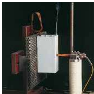
Apparatus for testing heat resistance (850° C) GWT.
