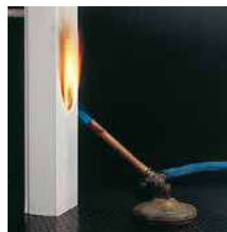
Apparatus for flame propagation resistance test.
