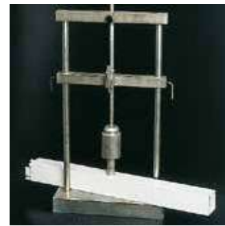
Apparatus for shock testing at low temperature.
